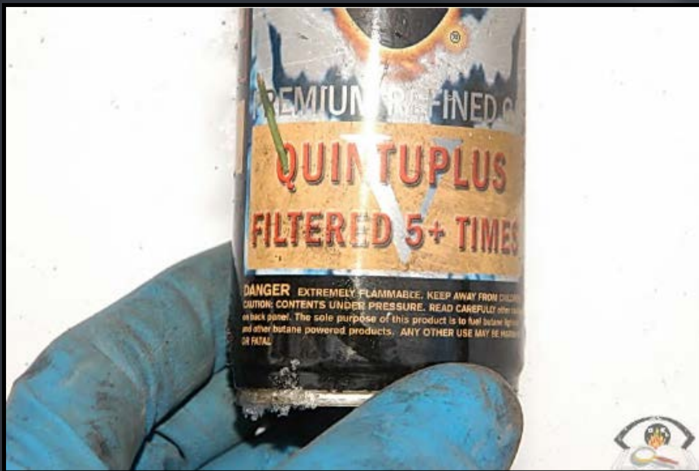
Image 6: A ruptured butane container was found approximately 13 feet from the exterior southeast side of the structure.
